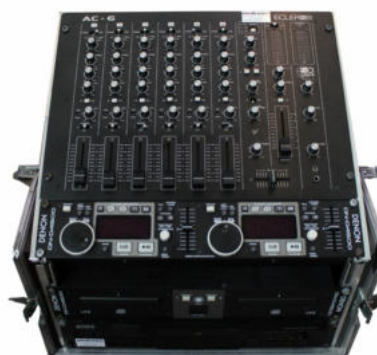
Discorack komplett (1 x DENON Doppel-CD Player D 4500, 1 x Discomixer Ecler/Soundcraft, 1 x Single CD-Player)
